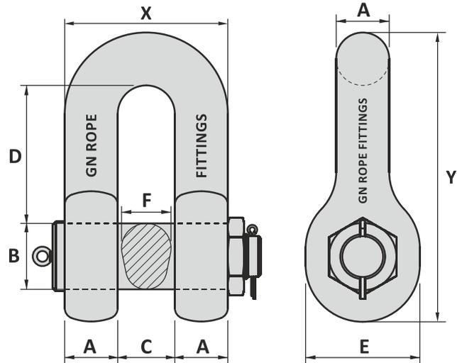
Dimensions for shackles are calculated by multiplying the common link size by the factor shown in this drawing.
