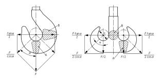
Skew loading shall be avoided by adjusting the rigging arrangement below the hook to allow the center of gravity of the load to line up with the centerline of the hook shank. The hook shall receive symmetrical vertical loads to minimize additional stress due to the bending of the hook shank.
