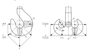
Skew loading shall be avoided by adjusting the rigging arrangement below the hook to allow the center of gravity of the load to line up with the centerline of the hook shank. The hook shall receive symmetrical vertical loads to minimize additional stress due to the bending of the hook shank.
