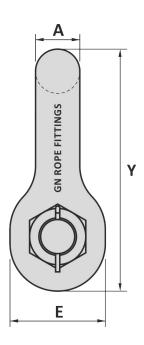
Dimensions for shackles are calculated by multiplying the common link size by the factor shown below
