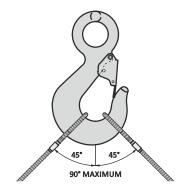
Never side load, back load or tip load a hook.
