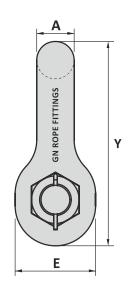
Dimensions for shackles are calculated by multiplying the common link size by the factor shown in this drawing.
